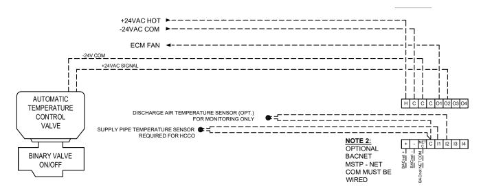
2-PIPE MODULATING HEATING OR COOLING WITH DISCHARGE AIR TEMPERATURE CONTROL, VARIABLE SPEED FAN SPEED FAN
